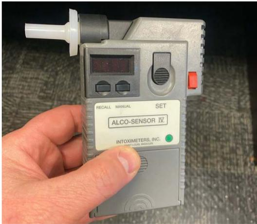
Running a Test - The Alco-Sensor IV product line has a one-way mouthpiece that is inserted into the instrument to turn the instrument on. The mouthpiece allows the subject to provide a sample for analysis. The mouthpiece is a large portion of the breath sample path, and the check valve in the mouthpiece reduces the likelihood that a subject will draw an inhaled breath sample, from the instrument, back through the mouthpiece.
