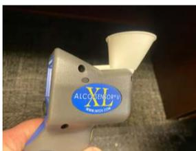
**Passive Testing** – A user should strongly consider whether or not they will use this method of testing. Given that there is uncontrolled breath being delivered towards the instrument, the ability of the operator to control where the breath goes is
