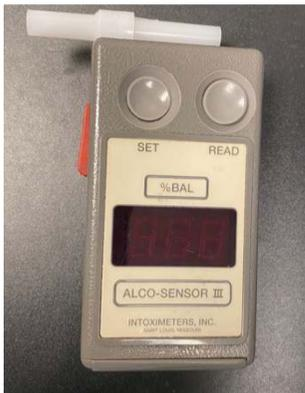
The Alco-Sensor and Alco-Sensor III product lines have a single nipple that the mouthpiece attaches to. The mouthpiece is effectively the entire sample path for the provided breath sample.
